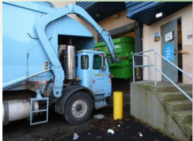
BINPAK is emptied and placed back on dock
